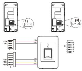
When using ProFP with Standalone access controller device, please move the dial code "1" to the ON position as shown above.
