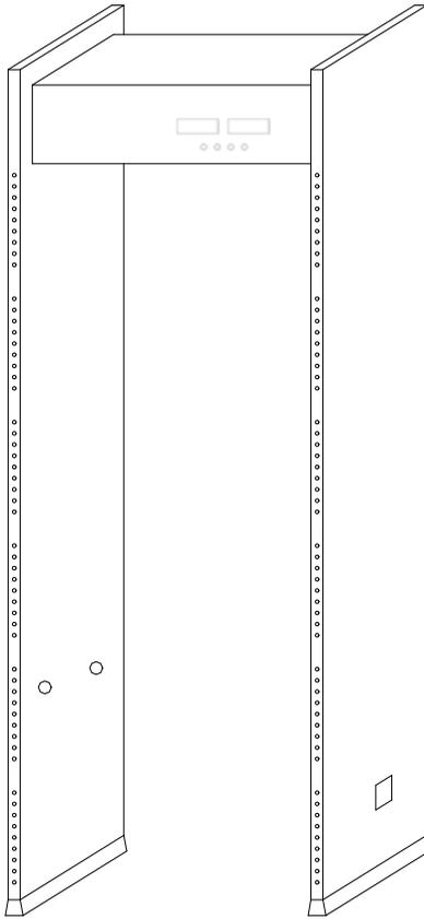
Walk Through Metal Detector is mainly used to check the metal items hidden on the body. When the passengers pass through the device, if they carried metals more than preset parameters value, the device would immediately alarms, and display alarm location, let the security guard find the people with the prohibited metal articles timely.
