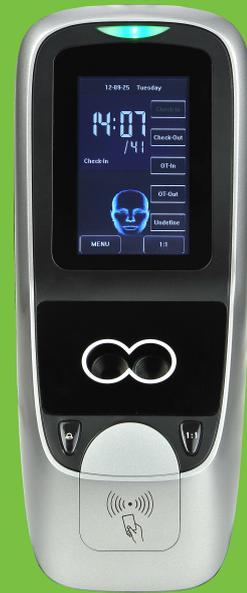
FAC700 is a new generation facial identification products, featuring standard functions with face recognition, PIN, and RFID verification. The unit encapsulates facial characteristics such as: relative position, size and shape of the eyes, nose, cheekbones, and the jaw features. All of these features are used for verification, and comparing with the enrollment data captured. The captured features are merged together into a value which are being compared to stored templates on the unit.
