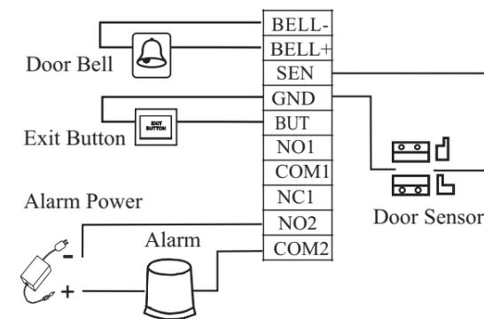
Alarm Voltage output  $\leq$  DC 12V
