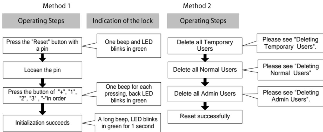
**Note:** The lock will be restored to factory defaults after initialization, and the door can be opened with any mifare card.
