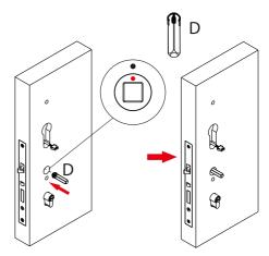
**Note:** Ensure the red dot have to be vertically upward.
