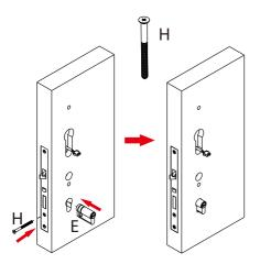
**Note:** Install lock cylinder in right direction, then tighten screw (H) to fix it.
