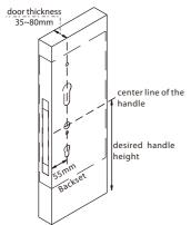
Note 1: Align the template along the vertical center line of the mortise (F) at the desired handle height, and tape it to door.
