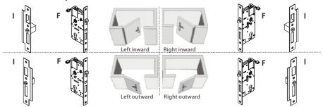
Note 1: Mortise (F) has 2 types: one is for left open, the other is for right open. Please use the correct one. Note 2: Strike plate (I) has 2 types: one is for inward open, the other is for outward open. Please use the correct one.
