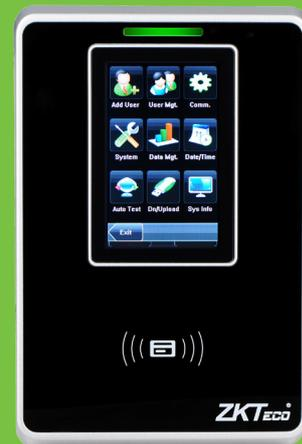
SC700 is a 125 KHz proximity access control terminal incorporated with 3" TFT LCD. The color display and touch screen operation offer a user-friendly and easy menu management.
